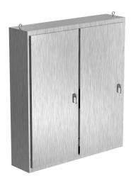
Saginaw NextGen series disconnect enclosure, NEMA 3R/4/4X/12/13, 86 x 78 x 18in (HxWxD), freestanding, 316 stainless steel, #4 brush finish, 2-door, 3-point padlocking combo handle.
