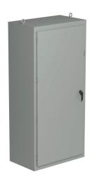
Saginaw NextGen series disconnect enclosure, NEMA 3R/4/12/13,  $86 \times 40 \times 24$ in (HxWxD), freestanding, carbon steel, ANSI 61 gray, polyester powder coat finish, single-door, 3-point padlocking combo handle.
