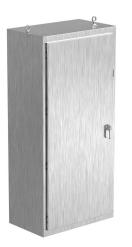
Saginaw NextGen series disconnect enclosure, NEMA 3R/4/4X/12/13, 86 x 40 x 24in (HxWxD), freestanding, 316 stainless steel, #4 brush finish, single-door, 3-point padlocking combo handle.
