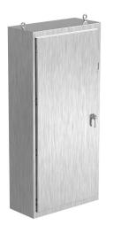
Saginaw NextGen series disconnect enclosure, NEMA 3R/4/4X/12/13, 86 x 40 x 18in (HxWxD), freestanding, 316 stainless steel, #4 brush finish, single-door, 3-point padlocking combo handle.
