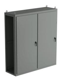
Saginaw NextGen series right disconnect enclosure bay, NEMA 3R/4/12/13, 86 x 78 x 24in (HxWxD), freestanding, carbon steel, ANSI 61 gray, polyester powder coat finish, 2-door, 3-point padlocking combo handle.
