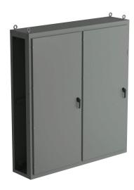
Saginaw NextGen series right disconnect enclosure bay, NEMA 3R/4/12/13, 86 x 78 x 18in (HxWxD), freestanding, carbon steel, ANSI 61 gray, polyester powder coat finish, 2-door, 3-point padlocking combo handle.
