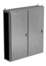
Saginaw NextGen series right disconnect enclosure bay, NEMA 3R/4/4X/12/13,  $86 \times 78 \times 18$  in (HxWxD), freestanding, 304 stainless steel, #4 brush finish, 2-door, 3-point padlocking combo handle.
