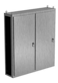
Saginaw NextGen series right disconnect enclosure bay, NEMA 3R/4/4X/12/13, 86 x 78 x 18in (HxWxD), freestanding, 316 stainless steel, #4 brush finish, 2-door, 3-point padlocking combo handle.
