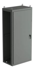
Saginaw NextGen series right disconnect enclosure bay, NEMA 3R/4/12/13, 86 x 40 x 24in (HxWxD), freestanding, carbon steel, ANSI 61 gray, polyester powder coat finish, single-door, 3-point padlocking combo handle.
