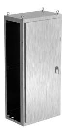
Saginaw NextGen series right disconnect enclosure bay, NEMA 3R/4/4X/12/13, 86 x 40 x 24in (HxWxD), freestanding, 304 stainless steel, #4 brush finish, single-door, 3-point padlocking combo handle.
