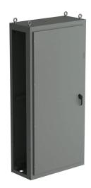
Saginaw NextGen series right disconnect enclosure bay, NEMA 3R/4/12/13, 86 x 40 x 18in (HxWxD), freestanding, carbon steel, ANSI 61 gray, polyester powder coat finish, single-door, 3-point padlocking combo handle.
