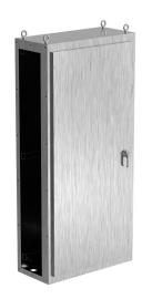
Saginaw NextGen series right disconnect enclosure bay, NEMA 3R/4/4X/12/13, 86 x 40 x 18in (HxWxD), freestanding, 316 stainless steel, #4 brush finish, single-door, 3-point padlocking combo handle.
