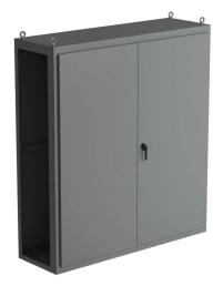
Saginaw NextGen series right enclosure bay, NEMA 3R/12/13, 86 x 78 x 24in (HxWxD), freestanding, carbon steel, ANSI 61 gray, polyester powder coat finish, overlapping double-door, 3-point padlocking combo handle.
