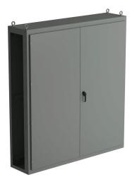
Saginaw NextGen series right enclosure bay, NEMA 3R/12/13, 86 x 78 x 18in (HxWxD), freestanding, carbon steel, ANSI 61 gray, polyester powder coat finish, overlapping double-door, 3-point padlocking combo handle.
