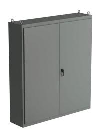
Saginaw NextGen series left enclosure bay, NEMA 3R/12/13, 86 x 78 x 18in (HxWxD), freestanding, carbon steel, ANSI 61 gray, polyester powder coat finish, overlapping double-door, 3-point padlocking combo handle.
