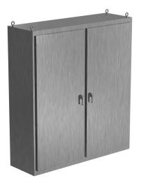
Saginaw NextGen series left enclosure bay, NEMA 3R/4/4X/12/13, 86 x 78 x 24in (HxWxD), freestanding, 304 stainless steel, #4 brush finish, 2-door, 3-point padlocking combo handle.
