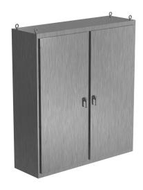
Saginaw NextGen series left enclosure bay, NEMA 3R/4/4X/12/13, 86 x 78 x 24in (HxWxD), freestanding, 316 stainless steel, #4 brush finish, 2-door, 3-point padlocking combo handle.
