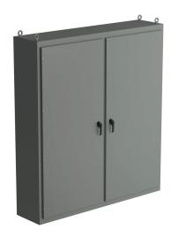
Saginaw NextGen series left enclosure bay, NEMA 3R/4/12/13, 86 x 78 x 18in (HxWxD), freestanding, carbon steel, ANSI 61 gray, polyester powder coat finish, 2-door, 3-point padlocking combo handle.
