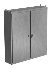
Saginaw NextGen series left enclosure bay, NEMA 3R/4/4X/12/13,  $86 \times 78 \times 18$  in (HxWxD), freestanding, 316 stainless steel, #4 brush finish, 2-door, 3-point padlocking combo handle.
