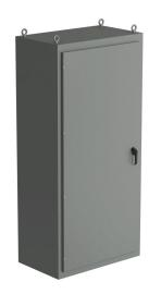
Saginaw NextGen series left enclosure bay, NEMA 3R/4/12/13, 86 x 40 x 24in (HxWxD), freestanding, carbon steel, ANSI 61 gray, polyester powder coat finish, single-door, 3-point padlocking combo handle.
