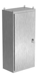
Saginaw NextGen series left enclosure bay, NEMA 3R/4/4X/12/13, 86 x 40 x 24in (HxWxD), freestanding, 316 stainless steel, #4 brush finish, single-door, 3-point padlocking combo handle.
