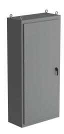
Saginaw NextGen series left enclosure bay, NEMA 3R/4/12/13, 86 x 40 x 18in (HxWxD), freestanding, carbon steel, ANSI 61 gray, polyester powder coat finish, single-door, 3-point padlocking combo handle.
