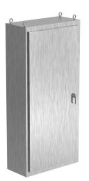
Saginaw NextGen series left enclosure bay, NEMA 3R/4/4X/12/13, 86 x 40 x 18in (HxWxD), freestanding, 316 stainless steel, #4 brush finish, single-door, 3-point padlocking combo handle.
