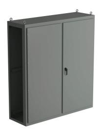
Saginaw NextGen series center enclosure bay, NEMA 3R/12/13, 86 x 78 x 24in (HxWxD), freestanding, carbon steel, ANSI 61 gray, polyester powder coat finish, overlapping double-door, 3-point padlocking combo handle.
