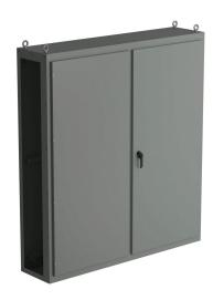
Saginaw NextGen series center enclosure bay, NEMA 3R/12/13, 86 x 78 x 18in (HxWxD), freestanding, carbon steel, ANSI 61 gray, polyester powder coat finish, overlapping double-door, 3-point padlocking combo handle.
