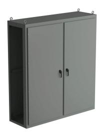
Saginaw NextGen series center enclosure bay, NEMA 3R/4/12/13, 86 x 78 x 24in (HxWxD), freestanding, carbon steel, ANSI 61 gray, polyester powder coat finish, 2-door, 3-point padlocking combo handle.
