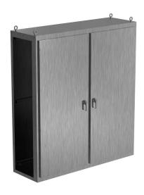
Saginaw NextGen series center enclosure bay, NEMA 3R/4/4X/12/13, 86 x 78 x 24in (HxWxD), freestanding, 304 stainless steel, #4 brush finish, 2-door, 3-point padlocking combo handle.
