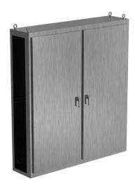
Saginaw NextGen series center enclosure bay, NEMA 3R/4/4X/12/13, 86 x 78 x 18in (HxWxD), freestanding, 304 stainless steel, #4 brush finish, 2-door, 3-point padlocking combo handle.
