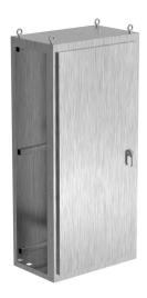
Saginaw NextGen series center enclosure bay, NEMA 3R/4/4X/12/13, 86 x 40 x 24in (HxWxD), freestanding, 304 stainless steel, #4 brush finish, single-door, 3-point padlocking combo handle.
