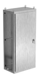
Saginaw NextGen series center enclosure bay, NEMA 3R/4/4X/12/13, 86 x 40 x 24in (HxWxD), freestanding, 316 stainless steel, #4 brush finish, single-door, 3-point padlocking combo handle.
