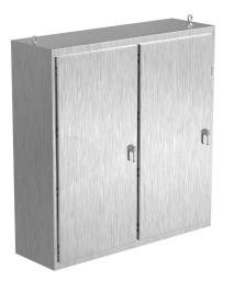
Saginaw NextGen series disconnect enclosure, NEMA 3R/4/4X/12/13, 80 x 78 x 24in (HxWxD), freestanding, 316 stainless steel, #4 brush finish, 2-door, 3-point padlocking combo handle.
