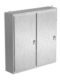
Saginaw NextGen series disconnect enclosure, NEMA 3R/4/4X/12/13, 80 x 78 x 18in (HxWxD), freestanding, 304 stainless steel, #4 brush finish, 2-door, 3-point padlocking combo handle.
