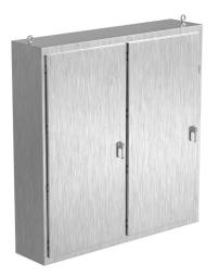
Saginaw NextGen series disconnect enclosure, NEMA 3R/4/4X/12/13, 80 x 78 x 18in (HxWxD), freestanding, 316 stainless steel, #4 brush finish, 2-door, 3-point padlocking combo handle.
