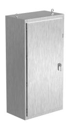
Saginaw NextGen series disconnect enclosure, NEMA 3R/4/4X/12/13, 80 x 40 x 24in (HxWxD), freestanding, 316 stainless steel, #4 brush finish, single-door, 3-point padlocking combo handle.
