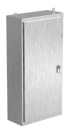
Saginaw NextGen series disconnect enclosure, NEMA 3R/4/4X/12/13, 80 x 40 x 18in (HxWxD), freestanding, 316 stainless steel, #4 brush finish, single-door, 3-point padlocking combo handle.
