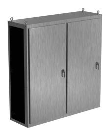
Saginaw NextGen series right disconnect enclosure bay, NEMA 3R/4/4X/12/13,  $80 \times 78 \times 24$  in (HxWxD), freestanding, 304 stainless steel, #4 brush finish, 2-door, 3-point padlocking combo handle.
