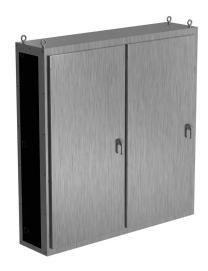
Saginaw NextGen series right disconnect enclosure bay, NEMA 3R/4/4X/12/13,  $80 \times 78 \times 18$  in (HxWxD), freestanding, 304 stainless steel, #4 brush finish, 2-door, 3-point padlocking combo handle.
