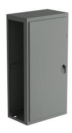
Saginaw NextGen series right disconnect enclosure bay, NEMA 3R/4/12/13, 80 x 40 x 24in (HxWxD), freestanding, carbon steel, ANSI 61 gray, polyester powder coat finish, single-door, 3-point padlocking combo handle.
