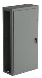
Saginaw NextGen series right disconnect enclosure bay, NEMA 3R/4/12/13, 80 x 40 x 18in (HxWxD), freestanding, carbon steel, ANSI 61 gray, polyester powder coat finish, single-door, 3-point padlocking combo handle.
