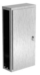
Saginaw NextGen series right disconnect enclosure bay, NEMA 3R/4/4X/12/13, 80 x 40 x 18in (HxWxD), freestanding, 304 stainless steel, #4 brush finish, single-door, 3-point padlocking combo handle.
