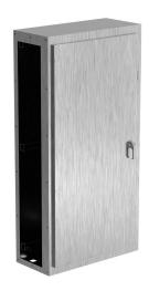
Saginaw NextGen series right disconnect enclosure bay, NEMA 3R/4/4X/12/13, 80 x 40 x 18in (HxWxD), freestanding, 316 stainless steel, #4 brush finish, single-door, 3-point padlocking combo handle.
