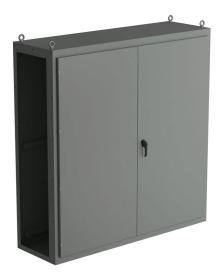
Saginaw NextGen series right enclosure bay, NEMA 3R/12/13, 80 x 78 x 24in (HxWxD), freestanding, carbon steel, ANSI 61 gray, polyester powder coat finish, overlapping double-door, 3-point padlocking combo handle.
