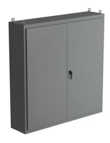
Saginaw NextGen series left enclosure bay, NEMA 3R/12/13,  $80 \times 78 \times 18$  in (HxWxD), freestanding, carbon steel, ANSI 61 gray, polyester powder coat finish, overlapping double-door, 3-point padlocking combo handle.
