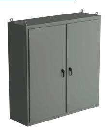
Saginaw NextGen series left enclosure bay, NEMA 3R/4/12/13,  $80 \times 78 \times 24$ in (HxWxD), freestanding, carbon steel, ANSI 61 gray, polyester powder coat finish, 2-door, 3-point padlocking combo handle.
