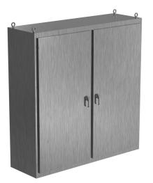
Saginaw NextGen series left enclosure bay, NEMA 3R/4/4X/12/13, 80 x 78 x 24in (HxWxD), freestanding, 304 stainless steel, #4 brush finish, 2-door, 3-point padlocking combo handle.
