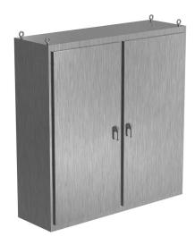
Saginaw NextGen series left enclosure bay, NEMA 3R/4/4X/12/13,  $80 \times 78 \times 24$  in (HxWxD), freestanding, 316 stainless steel, #4 brush finish, 2-door, 3-point padlocking combo handle.
