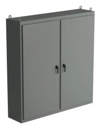
Saginaw NextGen series left enclosure bay, NEMA 3R/4/12/13, 80 x 78 x 18in (HxWxD), freestanding, carbon steel, ANSI 61 gray, polyester powder coat finish, 2-door, 3-point padlocking combo handle.
