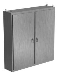
Saginaw NextGen series left enclosure bay, NEMA 3R/4/4X/12/13, 80 x 78 x 18in (HxWxD), freestanding, 304 stainless steel, #4 brush finish, 2-door, 3-point padlocking combo handle.
