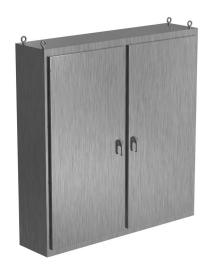
Saginaw NextGen series left enclosure bay, NEMA 3R/4/4X/12/13,  $80 \times 78 \times 18$  in (HxWxD), freestanding, 316 stainless steel, #4 brush finish, 2-door, 3-point padlocking combo handle.
