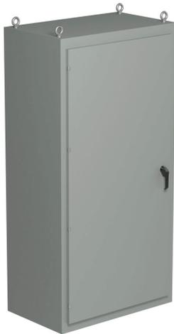
Saginaw NextGen series left enclosure bay, NEMA 3R/4/12/13, 80 x 40 x 24in (HxWxD), freestanding, carbon steel, ANSI 61 gray, polyester powder coat finish, single-door, 3-point padlocking combo handle.
